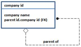
The recursive relationship for COMPANY includes the diamond symbol to indicate that the foreign key can be NULL, such as when a COMPANY has no parent. Recursive relationships must be both optional (diamond) and non-identifying.
