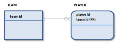
**Note:** Standard IE notation does not include rounded corners on entities. Rounded entity corners are an IDEF1X symbol included in IE notation to help ensure compatibility between methods.
